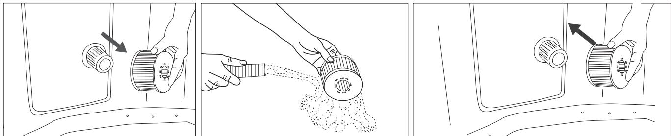
**NOTE:** Change the filter cartridge every 3-5 days, or if the filter cartridge remains soiled and discolored.
