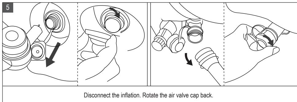
Disconnect the inflation. Rotate the air valve cap back.
