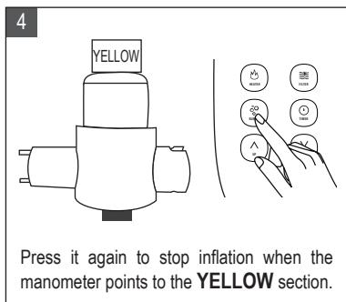
Press it again to stop inflation when the manometer points to the **YELLOW** section.
