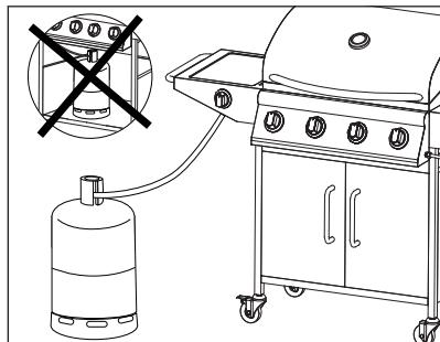
The designated space for storing the gas canister after use is: 71cm x 38cm x 49cm. In the event of a gas leak, turn off the gas supply.
