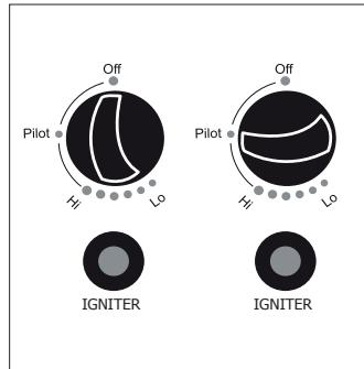
**!** **NOTE :** The burner may make a noise when it is first switched on. To eliminate this noise, turn the control knob to the pilot position. Then turn the knob back to the desired position.
