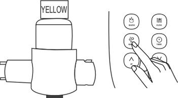
Press it again to stop inflation when the manometer points to the **YELLOW** section.
