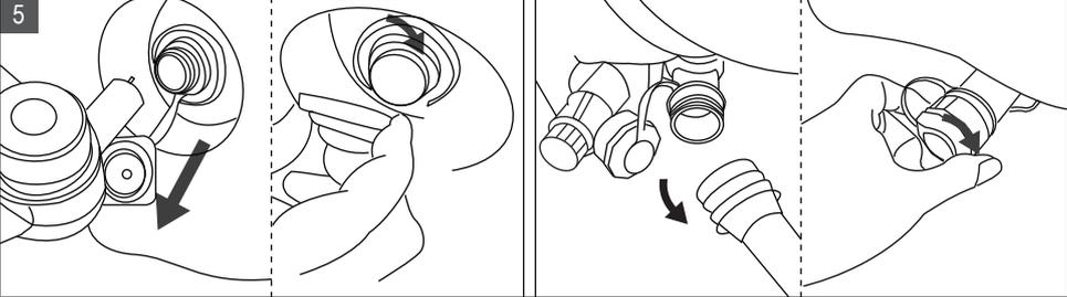
Disconnect the inflation. Rotate the air valve cap back.
