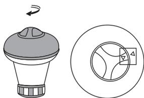
Rotate the upper cap counter-clockwise until two arrows meet. Remove the cap.
