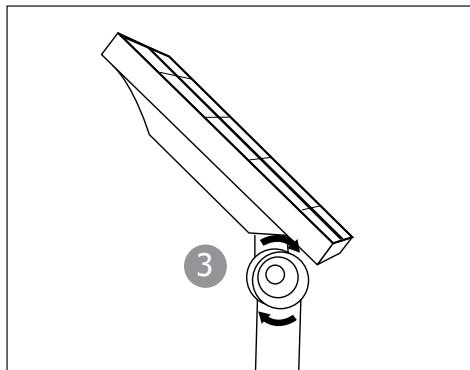
Make sure the solar panel is positioned to receive as much sunlight as possible. Take into account all obstacles to the light such as trees or buildings that might prevent a proper charging.
